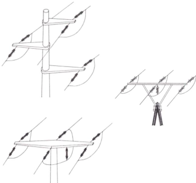
Strain poles with one conductor
